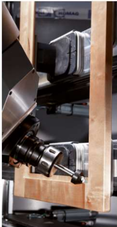
Square corner routing for a glass rebate
