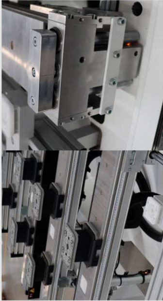
Solid Stop System (rear, side, front). Pneumatically lowerable solid stops incl. electronic end position monitoring
