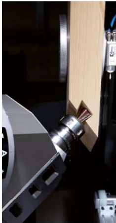
Routing of a dovetail joint for upright / transom constructions
