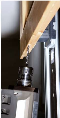
Step drilling for drill-in hinges
