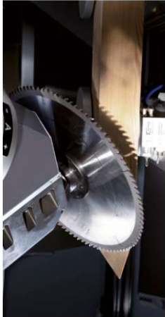
Mitre cut with high cutting depth for frames
