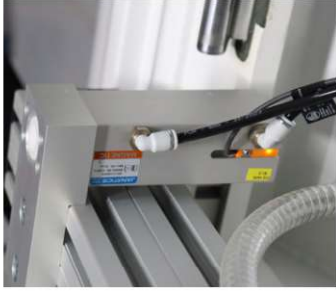
Electronic cylinder surveillance Enhanced security with the electronicsurveillance of lower cylinder positions at all integrated stops
