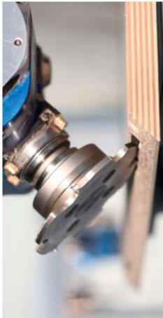
Cutting recesses for connecting fittings
