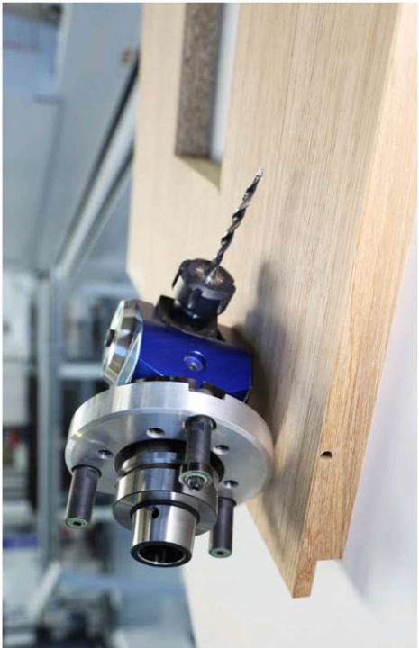
Holes for hinges Using the example of a door with rebate
