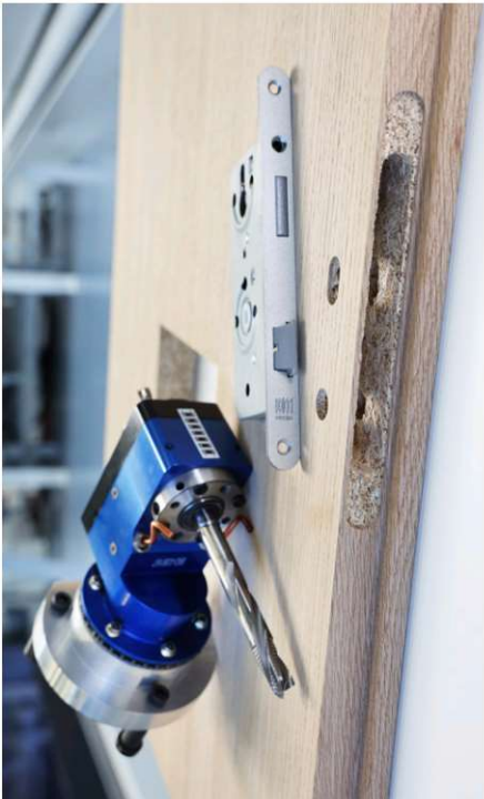
Lock case machining Using the example of a room door with a light cutout
