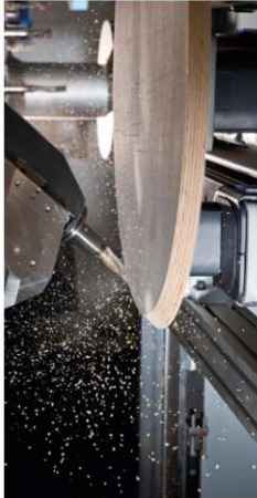
Chamfer trimming on a table top
