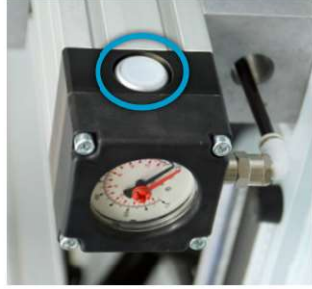
Button for program start Each one at the left and right hand stop profile act as program start for the processing.
