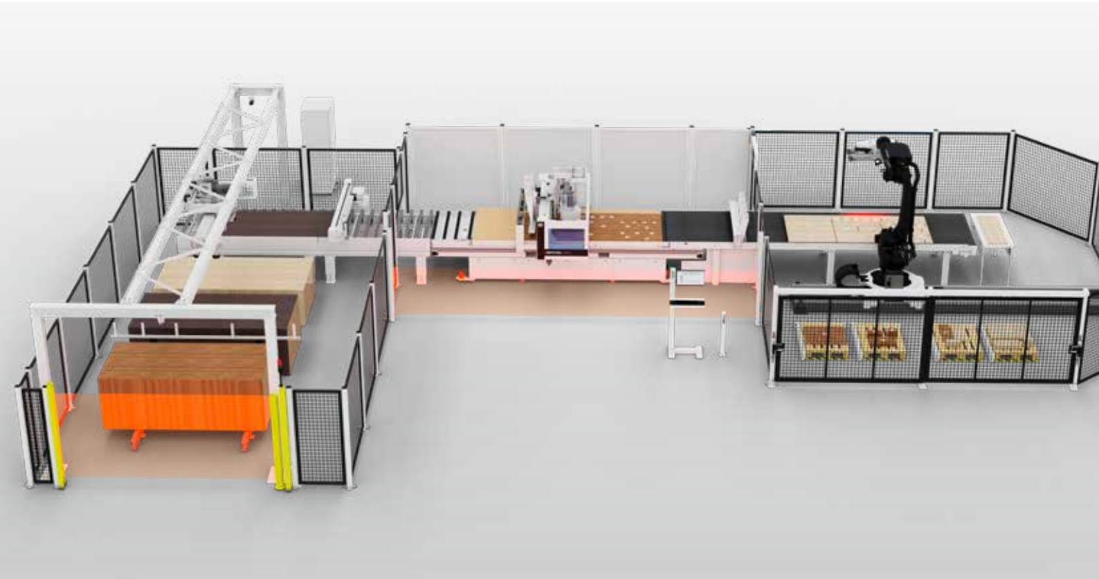
Including destacking via robot
