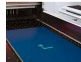
Rotation arrows on a workpiece show the required direction of rotation – until the alignment is correct.
