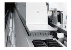
**Infeed stop**For minimum workpiece spacing and safe operation.
