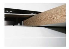
**Belt-type top pressure (optional)**Belt-type top pressure available as an option instead of the standard roller pressure system.
