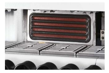
Workpiece pre-heating with heaters
