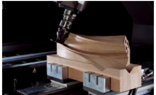
Routing a staircase handrail
