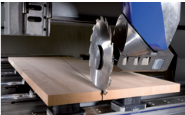
Separating cuts up to 110 mm in height
