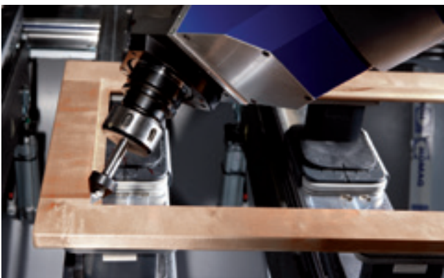
Angular cutting of a glass rabbet corner
