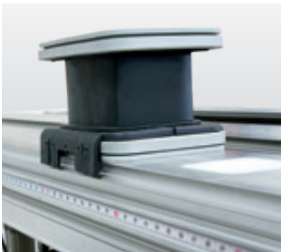
Measuring tape for positioning the suction units.
