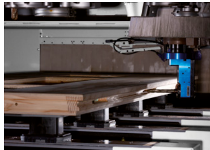
Lock case trimming on front doors
