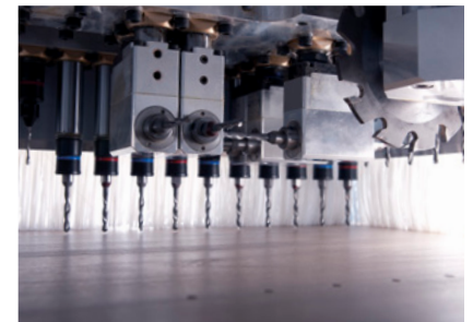
High-speed drilling technology with grooving saw
