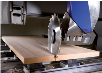
Dividing cuts up to 110 mm in height
