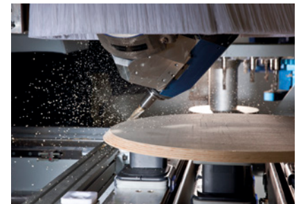
Chamfer trimming on a table top
