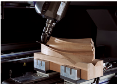
Routing of a stair hand rail
