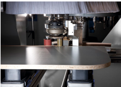
Gluing unit easyEdge for efficient banding onto shaped components
