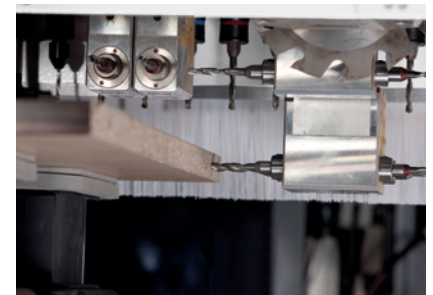
Horizontal boreholes for carcass connections
