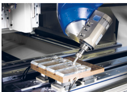
High-gloss trimming of acrylic parts
