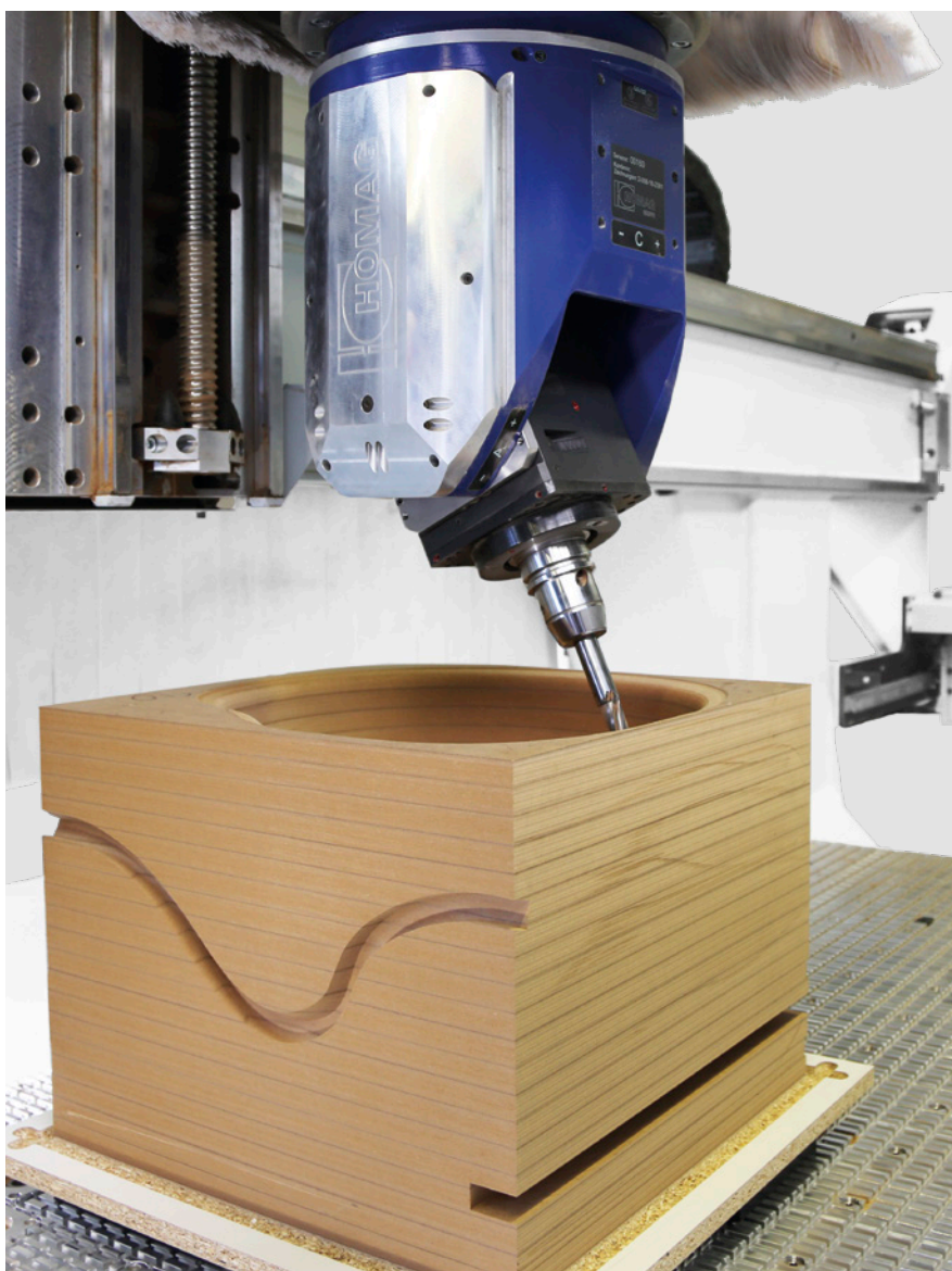
Trimming of components with large Z height
