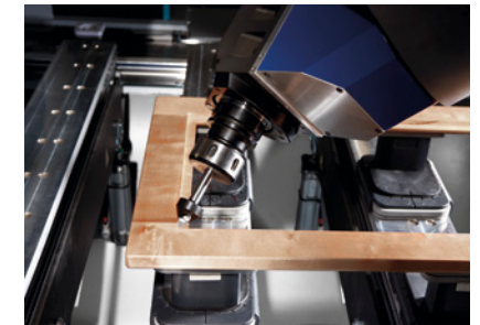
Square corner routing for a glass rebate
