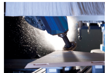
Trimming of inclined grooves for panel connection
